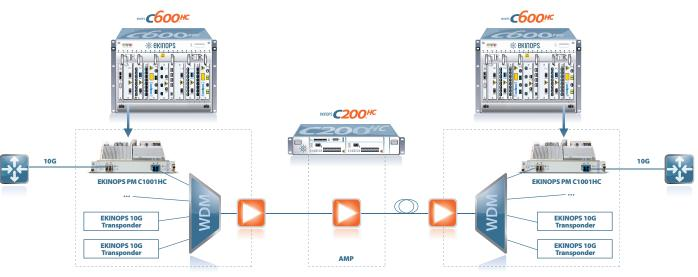
Up to 300 km without in-line Amplifiers More than 2000 km with in-line Amplifiers
